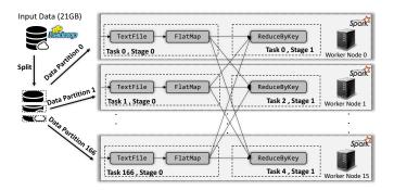
Figure 3: The physical execution of the motivating example by Apache Spark.
