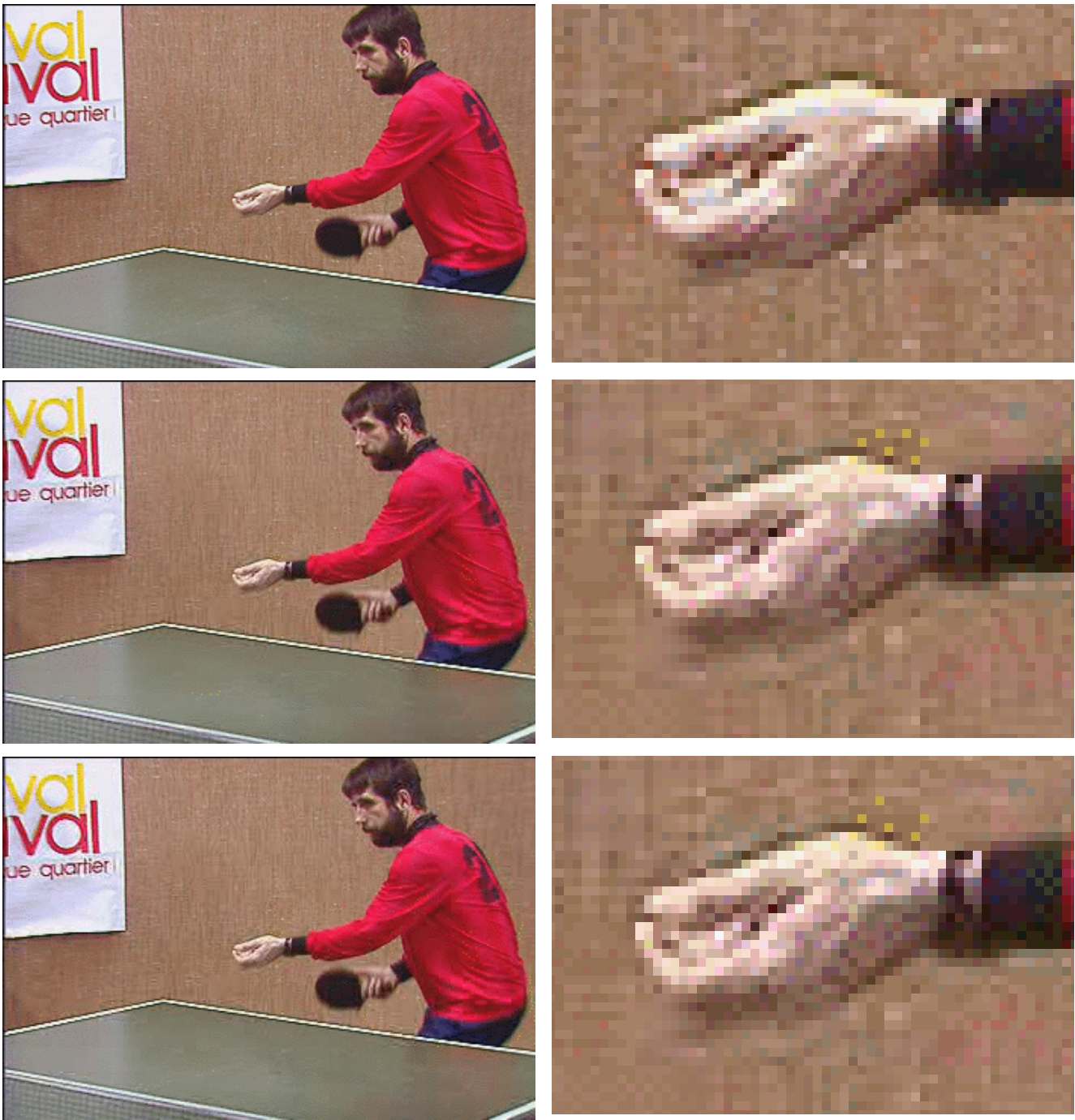
Fig. 15. Example for compressed-domain watermarking. Top: uncoded frame (sequence “table tennis”, CIF resolution), middle: MPEG-2 coded frame (2 Mbit/s) without watermark, bottom: the same MPEG-2 coded frame with embedded watermark (watermark amplitude 4).
